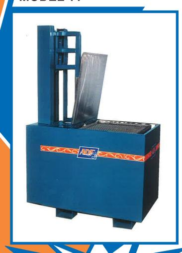
The ADF Dunker is a high quality parts washer utilizing aggressive agitation and dipping action for all types of parts washing. An optional pump agitation feature is available to speed up the cleaning action. The solution tank, platform and lift mechanism are constructed from 304 stainless steel. Dual double channel post provides a sturdy support and track for the lift mechanism.
